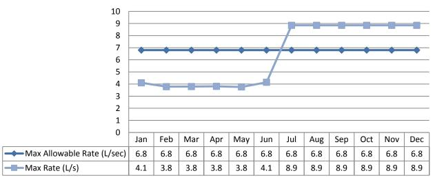
Note: The above table shows there were exceedances in instantaneous peak flow rate (L/s) this is due to well pump start-up and was not sustained. The actual limit in the PTTW is 409L/min. All spikes are reviewed for compliance.
